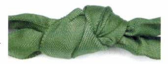
THE DAMAGE: Cuts to the cover NOT exposing internal core yarns –*Tuflex* roundslings all have a double walled jacket protecting the inner core yarns from damage. If damage (except for chemical or heat) appears only to the outer jacket and does not expose the inner core yarns, the sling may remain in service. To extend sling life, the sling may be returned to Lift-All for inspection and application of a patch to cover the damaged area.
